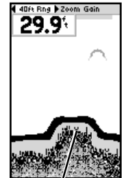
Structure is soft, probably a mud pile
